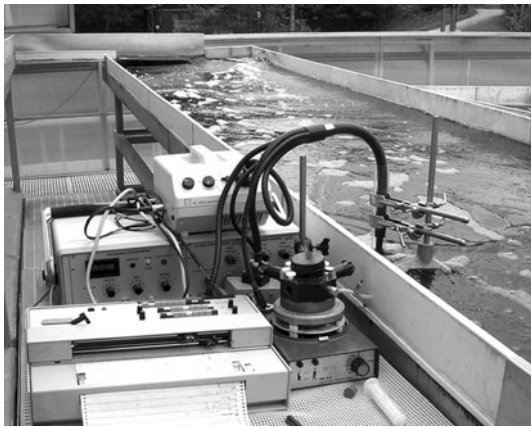
Fig. 3 In situ monitoring of Chl-fluorescence quenching using a fibre-optic guide and a pulse-amplitude-modulation fluorometer (PAM 101-103, H. Walz) connected to a recorder in the outdoor cascade units. The fibre-optics (angle to the sun being about 60°) was protected within a glass test tube and submerged about 3 mm into the microalgal suspension. Dark-adapted samples were measured in a stirred, temperature-controlled cuvette of the emitter-detector unit ED-101US (H. Walz, Germany) coupled to the fluorometer
